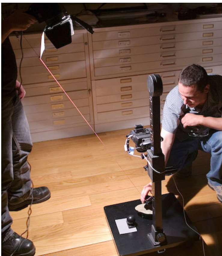
This camera is mounted on a copy stand, facing directly down onto the target object and spheres.
