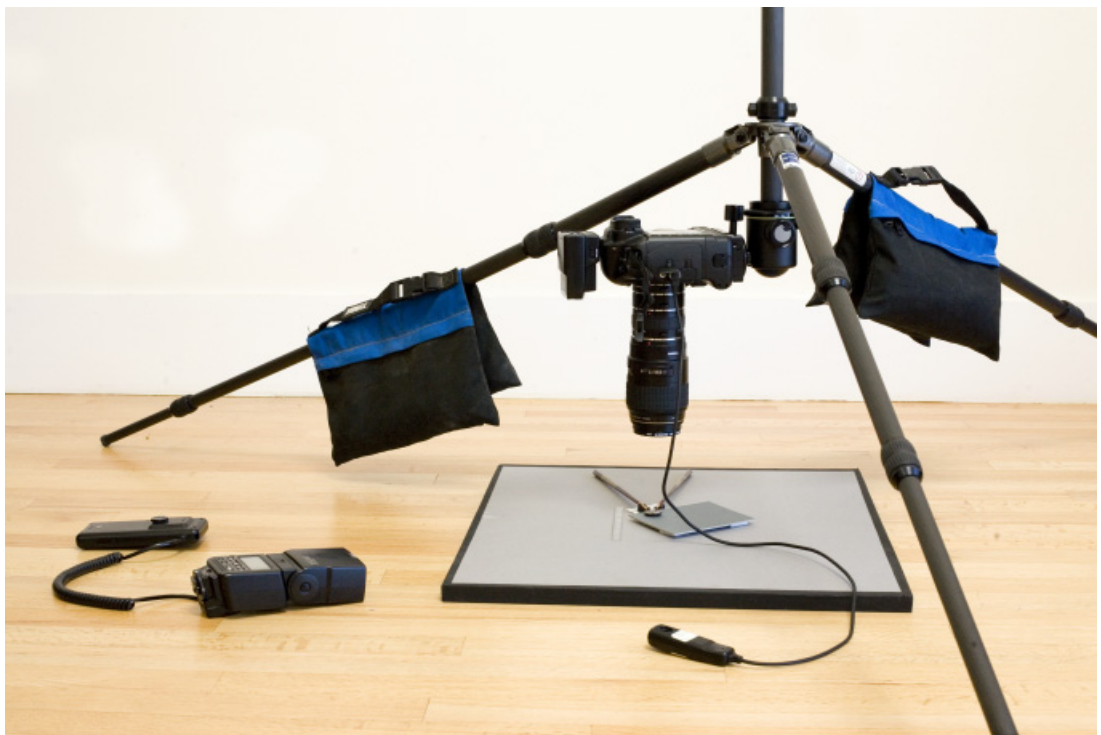
Camera attached to ball head fixed to bottom of central column of tripod, facing down
